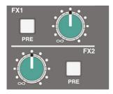
Note that it is possible to globally switch the FX Sends independently for the X-Panda to source the signal pre fader by engaging the "**PRE**" switch for either of the two FX Send busses on the last X-Panda Stereo Channel.
